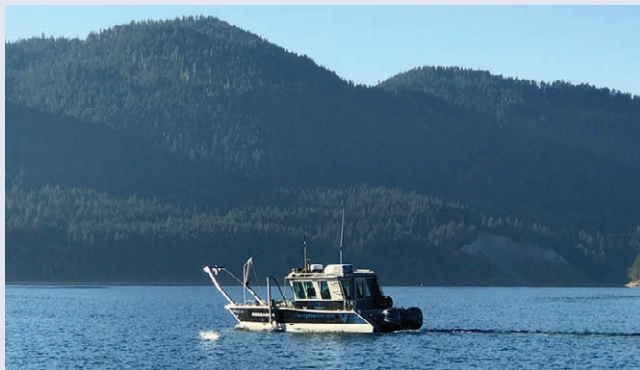
Specialized boat to support bathymetry
